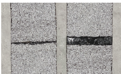
FIGURE 1: Too much bleed could be a sign of too much heat or the travel speed being too slow
