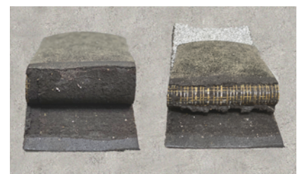
FIGURE 3: Underheated weld (left) compared with a properly-welded seam that separates at the scrim (right)
