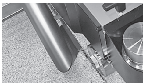
FIGURE 6: Slide nozzle head under seam
